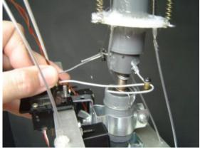
I'm using my hand to operate the head turning servo in the above pictures. This was easy to build and I may add another turning joint like this at the waist but it will be moving more weight so it has to be stronger.
