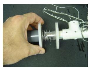
Heres how I plan on laying out this neck joint. I used a Hole saw to cut out my 3" plexi-glass disk. Then I used the center hole from the first 3" hole saw to use a smaller hole saw to cut out the middle. I did the same for the other disk but I used a different size hole saw for that center. I'm going to epoxy them together later.
