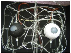
Above are pictures of the eyes. On the left is the back view and on the right is the front. I painted the eyes black first to prevent the red from the led from showing thru. After the black dries I paint it with white paint so when the led is on the red shows only thru the center of the eye. This makes the eye movement look really cool.
