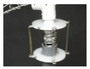
I used some wire to hold it in but its not going anywhere. On the right is the U Joint from Harbor Freight. The springs that are on the U joint help hold the head up pretty good.
