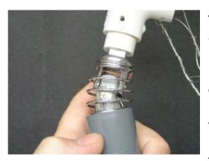
The neck is made up of a U joint with a 1/2" piece of pvc on the top that fits into the bottom of the 1/2" Tee. The bottom of the U joint fits in a 3/4" coupling that will connect to the 3/4" PVC pipe I'm using for a base. I have to make the two 3" round pieces of 1/4" plexi-glass to attach the springs too.
