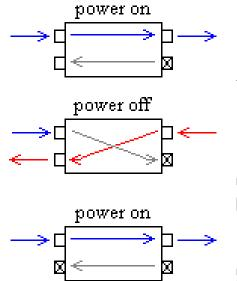
A four-way valve can act as a three-way by plugging one of the ports.
