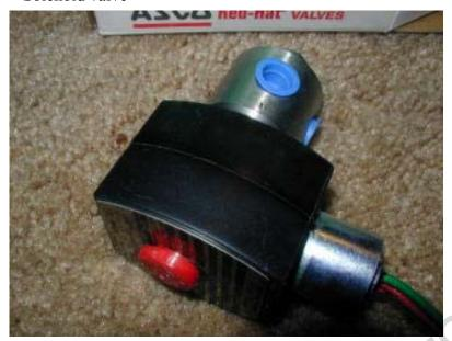
Each HAM has an electrically-controlled (solenoid) valve. It permits us to remotely cause air to flow from the storage tank to the prop. When we turn the valve back off, the air in the prop is expelled through the exhaust port.
