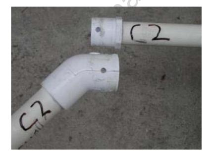
All of the leg sections are either glued or pinned.
