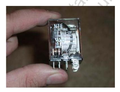
The relay used in this project is <u>Radio Shack</u> #275-217. It features a 110 VAC coil and DPDT contacts rated at 10 Amps. As of January 2002, it sells for \$7.99.
