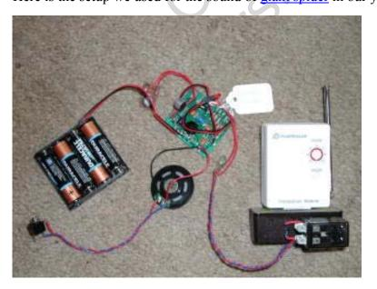
The <u>Radio Shack</u> recordable sound board is in the center. The <u>trigger relay</u> is lower right with the <u>X-10</u> module just above it. The wire from the sound board terminates in a 1/8" socket that connects to the <u>amplified</u> speakers.
