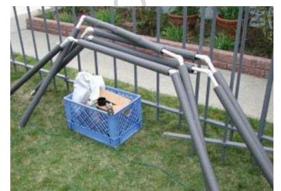
Each leg assembly takes little time: fit the three pieces of PVC together; pin the joints; cover with foam cylinder; pull cloth covering into place.
