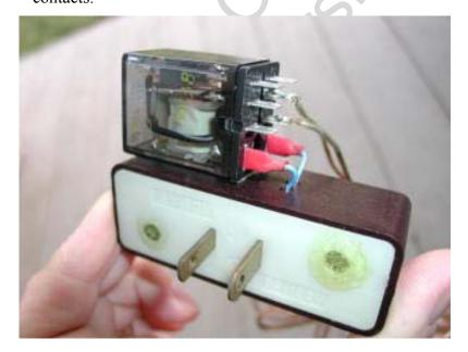
This is the completed trigger relay assembly.
