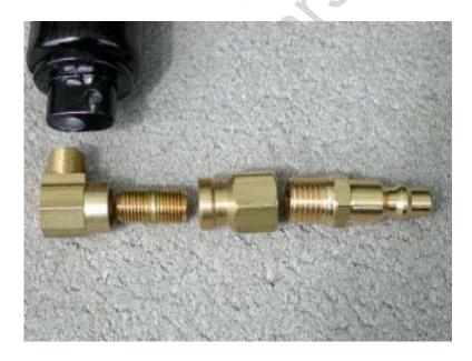
I rather like standard pipe fittings, so I'll be attaching this 90-degree elbow to the going into the door closer is 1/8-inch NPT cylinder. The threaded part that will be (National Pipe Thread).
