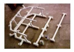
All of the parts are dry-fit. Only after everything is known to fit together properly is PVC cement used to permanently assemble the spider skeleton. The body will be glued up into a single unit. The legs are pinned into place, and can be removed and broken down for storage.
