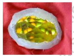
The spider was given a pair of eyes, made from faceted plastic "gems". Behind each gem was a pile of self-flashing LEDs, some yellow, some green. When activated, the LEDs twinkled, casting light through various facets.
