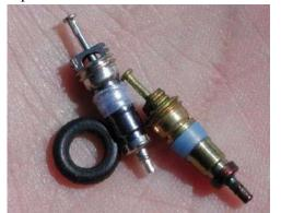
Both valves have removable spring "cores". Just unscrew them and they fall out. The valves cores themselves are similar to those used in automobile tires, and they unscrew the same way.
