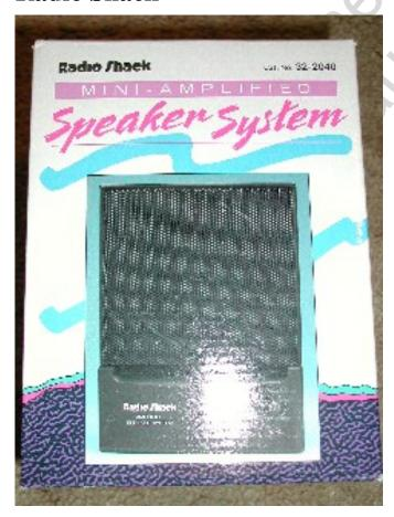
This is a little monophonic amplified speaker from Radio Shack. It is normally battery-powered, but has a jack to accept an external power source.
