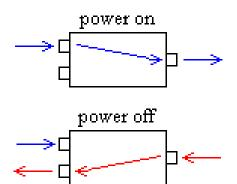
When power is on, one of the ports is connected to the common port, and pressure flows through to extend the pneumatic cylinder.
