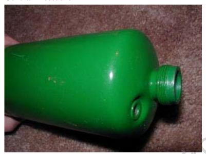
Construction is simple: get empty propane tank; make sure it's empty; unscrew and remove the two valves; wash out with soap and water; drill and tap for 1/4-inch NPT; clean; paint; replace the pressurerelief valve.
