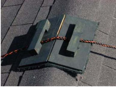
The base sits firmly on the roof. For added protection against sliding down the roof, a rope goes up, over the ridgeline, and fastens to a Heavy Object on the back side.
