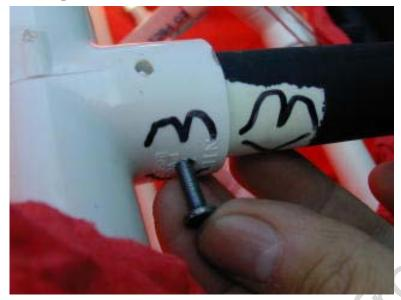
Each detachable piece is pressed together, and then fixed in place with a metal pin. A piece of masking tape around the piece keeps the pin in place.
