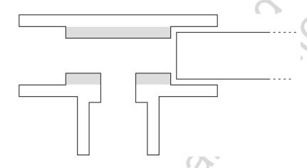
The standard PVC tee has a "shoulder" inside that keeps the pipe from being driven too deep into it. This is visible as the gray area in this cutaway view.
