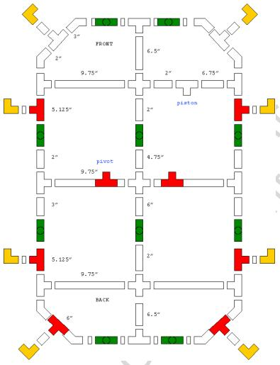
The bottom ring is composed almost entirely of 3/4" PVC. This is stronger material than is used in the upper ring. This is required because the lower ring does all the load-bearing.
