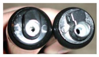
The hole for the valve screw is in two parts. The outer part is wide enough for the head of the screw to go in. The inner part is narrow, and threaded to accept the screw.
