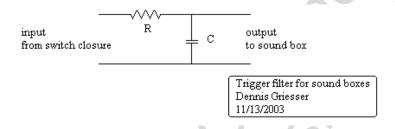
This is a simple low-pass filter. The cutoff frequency is given by:
