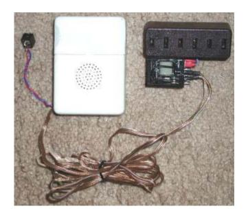
The canned scream is the big white box. The trigger relay is upper right. It is usually plugged into an X-10 module. The blue and red wires on the left from the sound box terminates in a 1/8" socket that connects to the amplified speakers.
