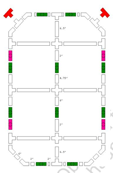
The upper ring is composed almost entirely of 1/2" PVC. This is lighter material than is used in the lower ring. This was done to reduce costs. We can get away with it because the lower ring does all the load-bearing. The upper ring just gives it rigidity and volume.
