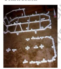
The spider started with a skeleton for the body constructed of PVC pipe and fittings. The shape is a pair of octagons, squashed so that they are longer than they are wide. The lower octagon is structural - all of the legs hang off ot if. It is built of 3/4" PVC. The upper ring gives shape, thickness, and additional stability to the body. It is made from 1/2" PVC. The spider contains roughly \$50 worth of PVC.
