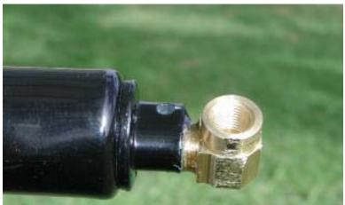
With a properly drilled and tapped hole, matching threads on the elbow, and epoxy, the result is quite strong.
