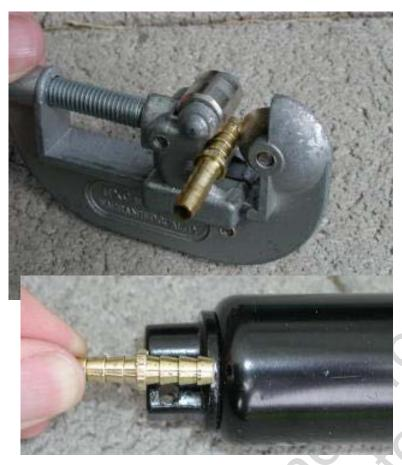
The simplest way to cut down the hose barb is with a pipe and tubing cutter. Failing that, use a hacksaw.
