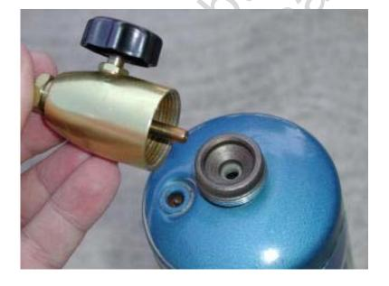
The center hold contains a check-valve that will only dispense propane when a properly designed appliance is screwed on.
