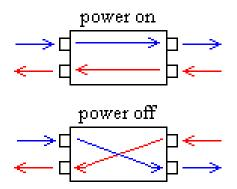
With power on, one set of ports is connected straight through to the other set of ports.
