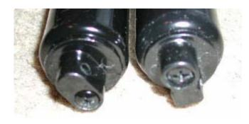
Find the air adjustment valve. It should be on the end of the cylinder body. It just looks like a screw. If you're lucky, it will be indicated by markings for "+" and "-" or "faster" and "slower". Most are unmarked.
