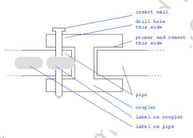
This is a cutaway view of a PVC coupler and the two pipes it joins.
