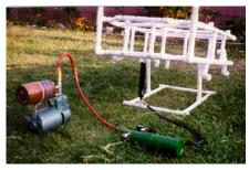
The spider is animated, because the only thing more terrifying than a giant spider is a giant spider lunging at you! The body is made to rock back and forth on a central pivot. Up front is an air cylinder that provides the motion. Although there is only one air cylinder in the spider, the rocking of the body causes all of the legs to move. When the spider lunges down at the victims, the front legs wave up and down.
