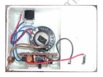
The final step is to drill a hole in the case and mount the socket. In operation, the amplified speakers plug in here.
