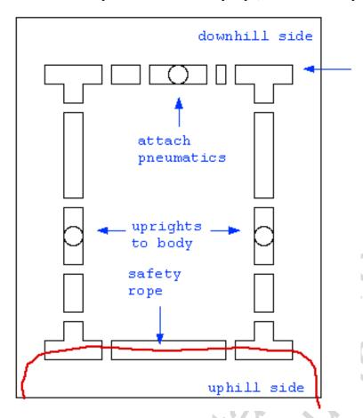
The PVC pipe provides attachment points for the spider and pneumatic cylinder. It also starts spreading the weight around. The safety rope is passed through the uphill PVC pipe. The spider spitter is attached to the downhill PVC.
