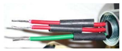
A solenoid valve that operates on 110 VAC line current may have three wires.
