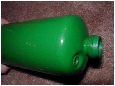
With a full order of HAM, you get Green Egg, the air storage tank made from a recycled propane tank. The compressor makes all the pressurized air that we need, but might be tempted to run its motor all night long. In order to keep the motor from running, we provide air storage tanks. The motor runs only until the storage tanks are filled, then shuts off until the storage tanks run low again.
