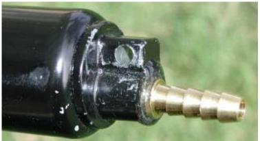
Make sure the hole and the hose barb are clean and grease-free! Then, epoxy the barb into the hole.
