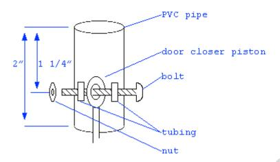
The top of the screen door closer is attached to the PVC with a movable link.
