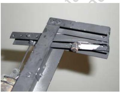
Attached to the lever is a bolt, sticking down, toward the can. The idea is that, if you were to pull the lever down towards the can, the bolt would press down on the nozzle, dispensing the cream, as if you had pressed the nozzle with your finger.
