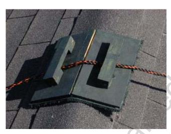
A PAIR of pads like these protect the roof against abrasion from the safety rope that keeps the spider from sliding down the roof.
