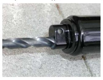
The threads in the inner hole are too small for the 1/8" NPT elbow. And the outer part of the hole isn't threaded at all, and makes a tight fit with the elbow.
