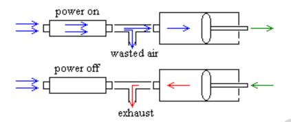
When power is applied, compressed air goes into the pneumatic cylinder, *and* escapes through the bleeder valve.
