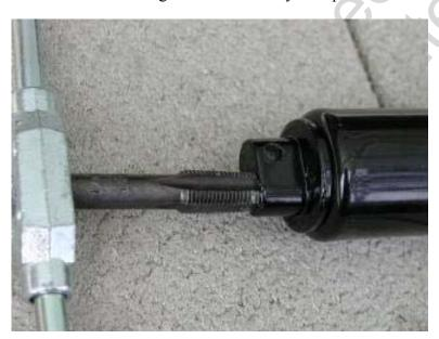
Tap the hole all the way through (inner and outer) with a 1/8" NPT tap.
