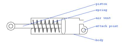
Cutaway view of a door closer.
