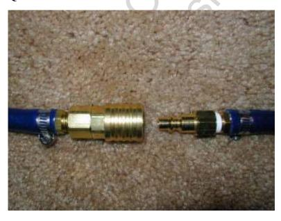
We like to give our components a common, standard connection. This allows us to move them around as required and replace tired units with spares. The snap-on air connectors are a key to this. Our compressor and all of our hoses and manifolds use these same quick connectors. Any time we want, we can add 50 feet of hose, a manifold, or another HAM - just by snapping it into place.
