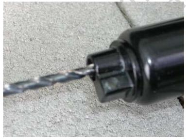
The inner threads in the hole are too small for the hose barb. The outer part of the hole is too large.
