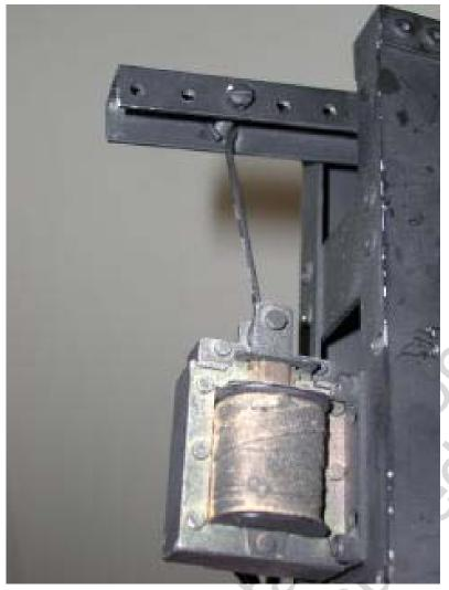
Parts are not critical, except that you get them to fit together. The solenoid is a 110 VAC pull model from the electronics junkbox. Leverage is used to give it strength, so it need not be particularly strong. Try the usual surplus stores: <u>Jameco</u>, Hosfelt, MPJ, All, Goldmine, Herbach.
