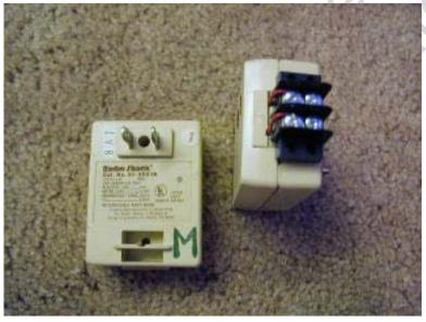
There are a lot of tricks you can do with X10. These appliance modules have been hacked. The one on the left is now momentary-activation. The one on the right has dry-contact output.
