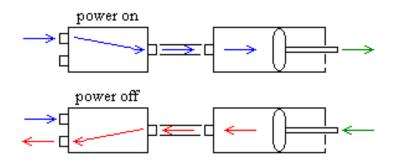
When power is applied, compressed air goes into the pneumatic cylinder, and only into the cylinder. No wasted air.
