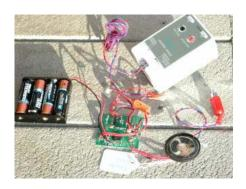
The <u>Radio Shack recordable sound board</u> is the green thing in the center. The X-10 relay module is in the upper right. The wire from the sound board terminates in a male RCA plug on the right that connects to the mixer on the sound system.
