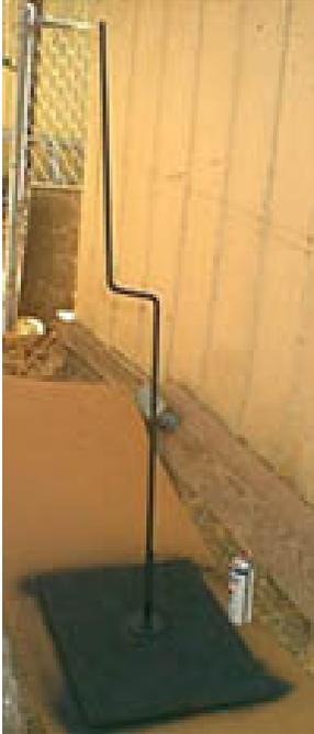
Clean the Steel Rod with soap and water to remove any oils that may prevent paint from sticking, then dry thoroughly. Spray paint the metal rod with flat black spray paint.
