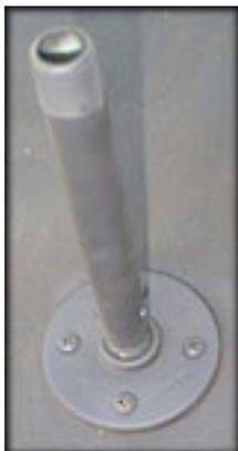
To make the base, find the center of the 2'x2' board you will be using and mark it. Place the Floor Flange in the center of the board and attach securely with four screws. Screw the 1/2"x8" pipe nipple into the floor flange until it is tight.
