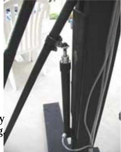
The linkage is extended by a pneumatic cylinder with a 10" throw. The cylinder is assisted by a 22 pound counter weight that hangs off the top tube.
