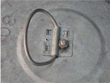
As purchased from the store, the handle for the trash can is merely crimped on the lid. To the left of center is a pop-rivet that helped hold things together during construction. To right of center is the threaded end of the bicycle tire pump, with a nut on the end.
