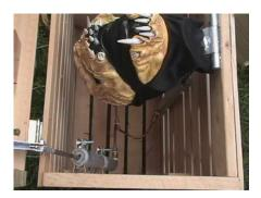
He used two screen door cylinders to build the prop: one that opens the crate lid, and the other to pop out the head. The head is a light, styrofoam wig head from Sally's Beauty Supply with a full head-cover mask over it. It is connected to the crate with a heavy-duty door hinge. Hence the popping out rather than up.
