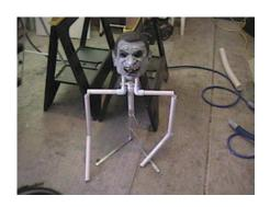
The original grave jumper I built was attached at the shoulders directly to the end of the piston. This simple design worked out pretty well, but didn't have a lot of throw (height).
