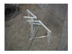
Here's a shot from the back (looking over the right shoulder). The top posts are a bit too horizontal in this picture. The head has smaller diameter PVC posts that slip inside the ends of the top pipes. A small screw through both pipes keep the head from flying off when the piston hits the top.
