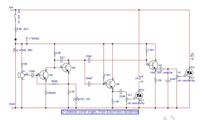
The sounds are detected by the FET microphone and amplified by transistors Q3 and Q4. Both channels take their driving signal from Q4, but through different value capacitors, which gives them their frequency sensitivity. Each channel has a driver transistor, which feeds a triac, which switches the load.
