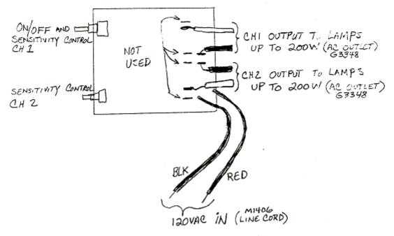
()ITS A GOOD IDEA TO ADD A SAMP FUSE IN SERIES WITH THE POWER INPUT RED LEAD
