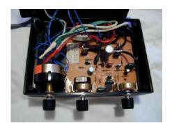
The top half of the control box contains the color organ board from Electronic Goldmine.
