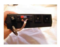
This is the back of the control box. It shows: fuse, speaker-level sound input, and a socket for the lamps on each channel.
