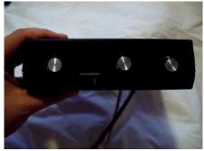
The front of the control box has: master level control, power switch, and individual level controls for each channel.
