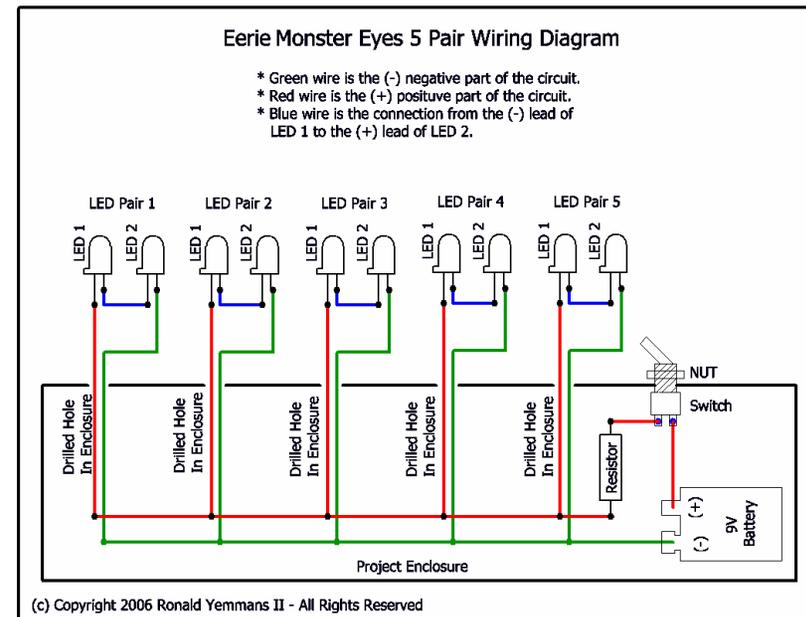
Note: These two circuits are functionally the same. The second circuit reduces the number of number of resistors from 5 down to 1. The important thing to realize here is that considerably more current is flowing through the single resistor and we need to be concerned with the **HEAT** that will build up in it.
