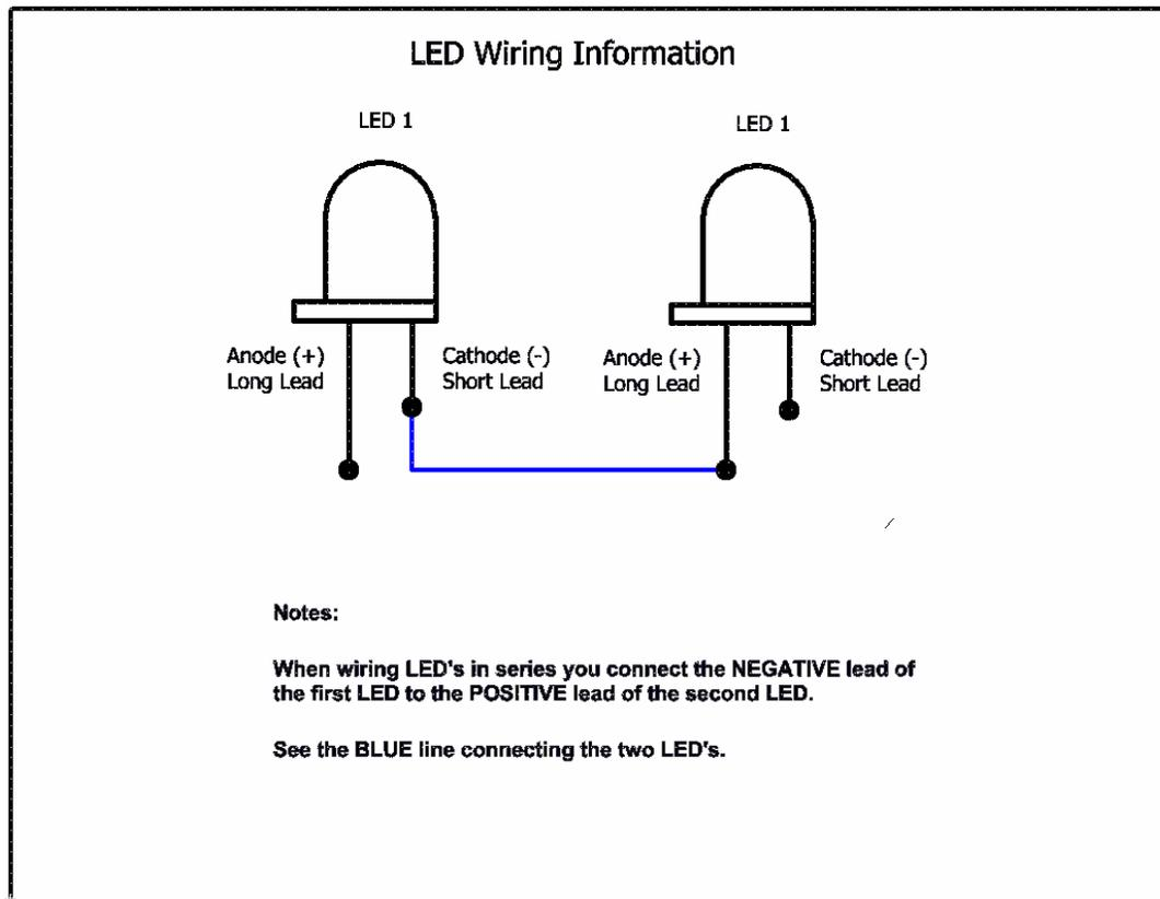
When connecting two LED's in series it is important to connect them properly. If you do not wire the LED's properly they will not light up and you might damage both LED's.
