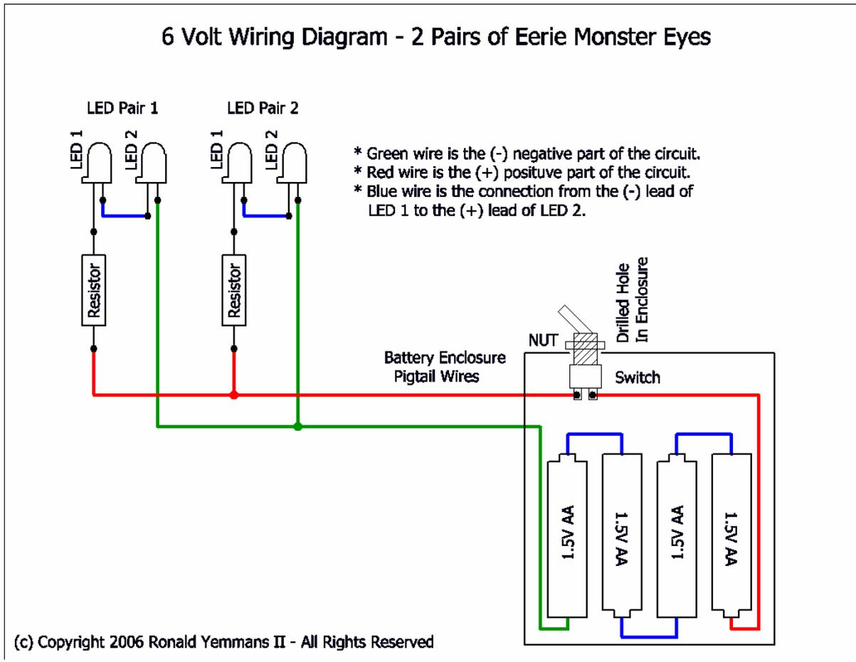
*Is there a difference in how this circuit works as compared to the circuit in Example 1?* Only a minor difference exists. This difference is that a total of **.040 amps** will be drawn from the batteries which will cause them to "die" twice as fast.
