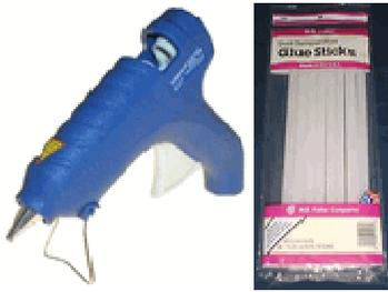
Glue gun for gluing the wires and resistor in the enclosure. The wires are glued to help prevent them from being pulled out of the box.
