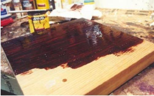
After the hole is drilled you will need to paint or stain the wood mount. I used red oak wood stain. Make sure to get it down the hole you just drilled.
