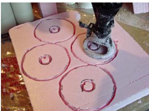
*Cut out the centers first and push out. Then cut out the circles and separate. I used a Dremel with the small router attachment multi-purpose cutting bit.*
