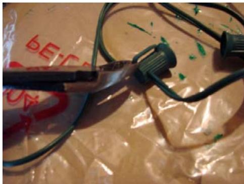
*Snip off the clip on the side of the socket. If you need to extend the wire length, you need to make sure you make water-proof connections. Since I'm not an electrician and I'm just guessing how to do that, I'm not going to show how I made mine. I don't want to be responsible for anyone getting electrocuted, just myself. Sorry :(*
