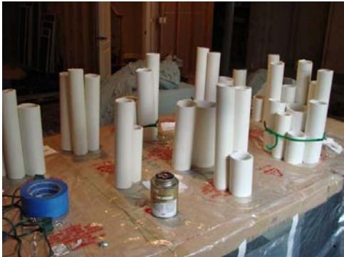
*Cut out PVC using either a PVC pipe cutter or circular saw. I hear the PVC pipe cutter is easier... :) Then glue your preferred arrangements using PVC glue. I had to re-glue a couple of times to have it hold.*
