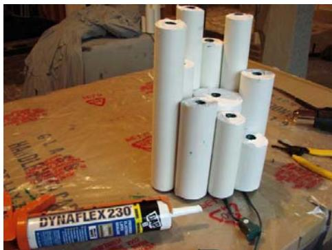
*I used caulk to cover up and seal the foam.*
