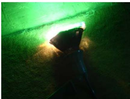
The picture on the left shows a standard flood light with a ground stake and a colorized gel taped to the front.
