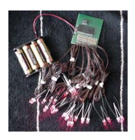
This is a little microcontroller circuit that has 15 pairs of L.E.D.'s that look like rodent eyes. The pairs of eyes blink in a semirandom fashion. So, what you end up with is 15 pairs of eyes staring out at you with one pair blinking (looks like the animal had to close their eyes briefly) at a time. The pairs of eyes are on wires so that they can be placed around the cave, bushes, etc. Runs off of 4 AA batteries.
