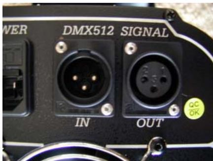
Here are the connectors on the back of an ADJ X-Cess fixture. Note that it is equipped with both a DMX input and output.
