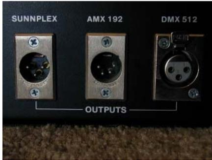
Here is the output of the Sunn PLC 3200 control console. It sends exactly the same information in three different formats (it also speaks MIDI). We are interested in the DMX output to the right.
