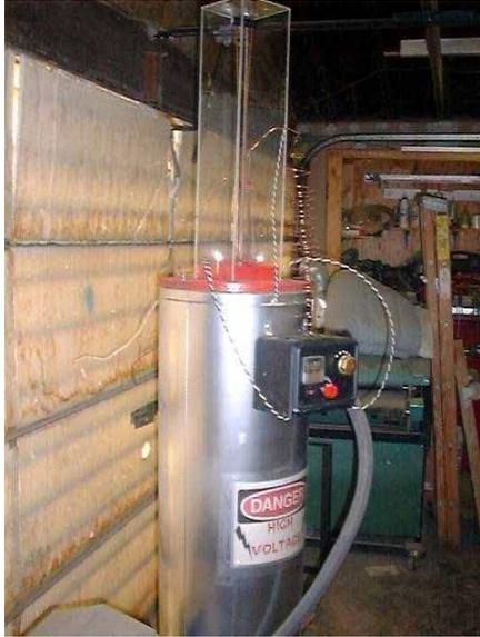
Then I attached a piece of 2 x 4 over this hole this is the mounting block for the Jacob's ladder wires. I used 8 gage wire for this about 30" long that are screwed into connector blocks on the 2 x 4 block. I painted this part red and made a Plexiglas box to fit over the Jacob's ladder. To weld the sides of this together I used my soldering iron and melted the pieces together with butt joints. Then this was screwed to the 2 x 4 block on top of the plywood.
