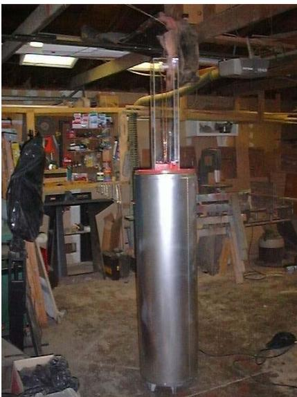
The first thing I did was to paint the outside of the water heater silver. I did 2 coats of paint on this but only used one can of paint as silver goes a long way. Then I cut a piece of 3/4" plywood for the top and cut a hole out of the middle for the flue pipe hole.
