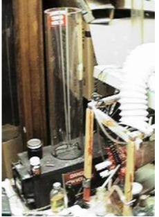
A 7,500 volt spark climbs an 18" Jacob's ladder making a nice "buzz.... pop!" sound. It's powered by a neon sign transformer bought at a surplus store for \$35. This is a *lethal* voltage/amperage. The spark will set a piece of paper on fire. The visitors are kept away from the table (for obvious reasons) by a metal mesh stapled to a wooden frame screwed into the doorway. The Jacob's ladder has a cooling fan on the side.
