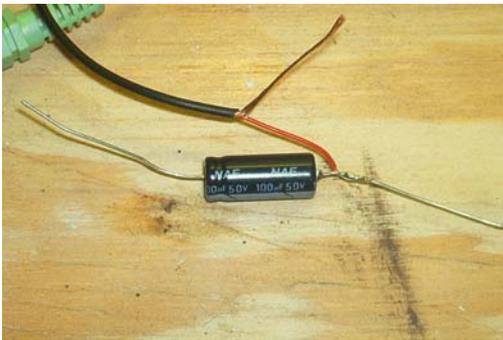
Twist the speaker wire from the powered speaker around the other lead on the capacitor (the wire with the insulation, not the bare copper wire), and solder this.
