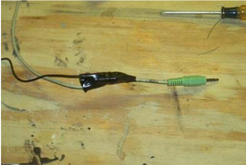
The end result is a single phone plug that splits into the lead that goes to the Boris, and the lead that goes to the speaker.
