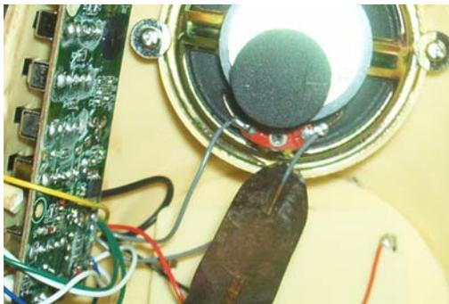
CAREFULLY strip about 1/2 inch from the 2 gray wires you just cut that are coming from the circuit board, NOT the wires from the speaker. To do this I grab the wire with needle nose pliers first, so that when you strip the wire you are pulling against the needle nose pliers, not where the wire is connected to the circuit board. You do not want to pull the speaker wire out of the circuit board.
