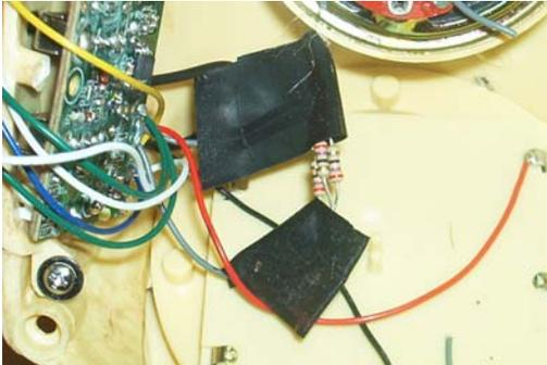
I use a little electrical tape to cover the bare wire on the resistor connected to the speaker leads, and the connections you made earlier with the speaker cable, capacitor and Boris microphone cord.
