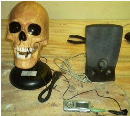
Here is everything you need for this project; A 100 microfarad capacitor, a 10 ohm resistor, a powered computer speaker, and a Boris. You will also need a music source you can plug the speaker into for testing
