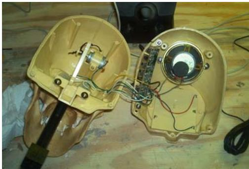
Carefully cut the 2 gray wires that go to the speaker, leaving about an inch of wire next to the speaker in case you want to connect the internal speaker back up.
