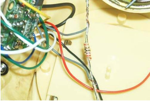
then wrap the striped end of the other gray wire around the other end of the resistor. Solder these connections.
