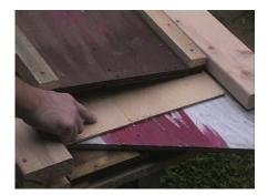
Then cut a 1/2"x 6" piece of wood. Mark 2" in on the bottom of both sides and cut on an angle to the top corner. Lay and square the board across the top face of the guillotine - screw in place.
