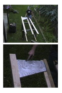
Make sure you have saw horses or something similar to work on. First, take two 2x4x8's and sandwich a 5/8x2x8 in between. Keep all three pieces flush to one side and close together. Fasten both sides with 2 and a half inch screws. I like to pre-drill the holes first as it makes things a lot easier.
