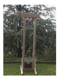
Leave enough room for the pulley plus 4" between the top of the blade and frame. When you have the blade where you want it, find the upper angle of the cutting edge. This will be the center mark of the hole you are going to make in the side of the blade track. Length of hole is about 4-1/2".
