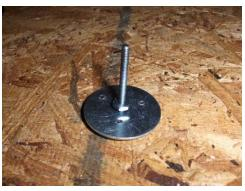
Install bolt and nuts so washer spins freely. Add Locktight so nuts do not tighten.
