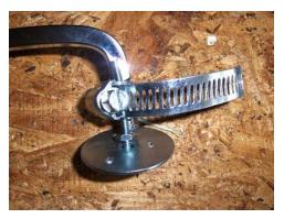
Attach assembly to shaft. This on only a dry fit you will need to remove to put through wooden frame later.
