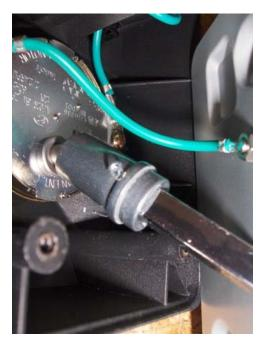
Open up the rotisserie so you can get ready to secure the shaft to be fixed to the motor.
