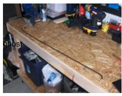
Bend shaft 90 degrees at motor and at other end. The rotisserie shaft is also too long so you will need to cut it off to your desired length. That will be determined by the size of your
