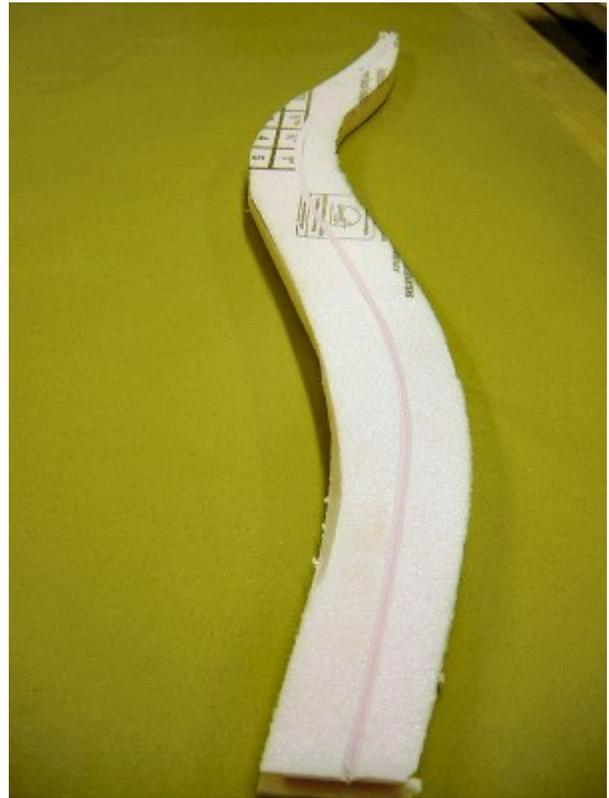
The Spine will be built using 3/4" extruded foam.
