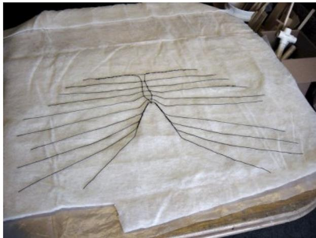
After the adhesive has dried, we used a 1" brush to paint the rib areas of the batting with liquid latex.
