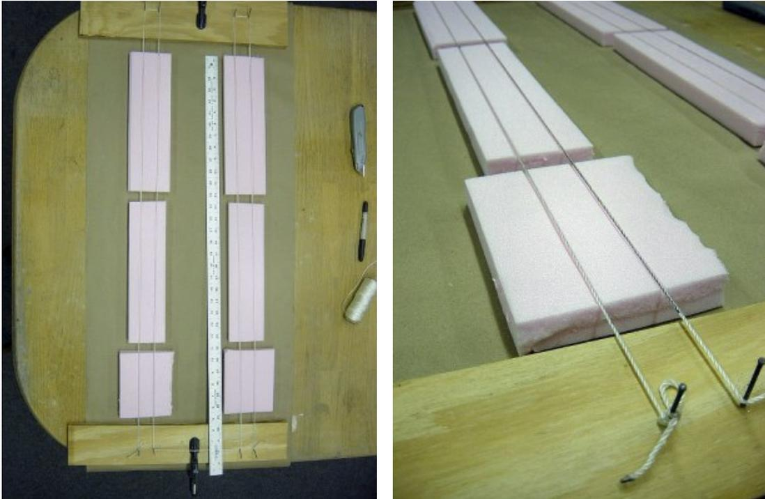
The arms for our Skeleton Marionette will be made using the same materials and construction techniques as the spine. Sheet foam is cut to approximate length and slightly excessive width.
