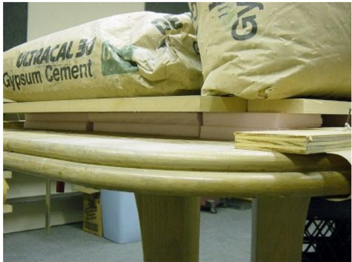
Same procedure ... apply a thin, even coat of polyutethane glue to one half of the joint and mist the other half with water. Place the twine in the grooves, assemble the halves, and clamp.
