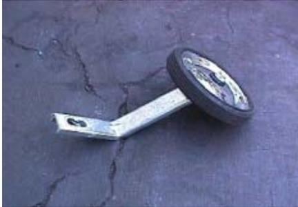
A metal training wheel is used as the motor's own drive wheel. When you first get the wheel there is a hard rubber wheel around the rim. If you have trouble prying it off....just pour some gasoline on it and it will burn itself into a crusty ash and then you chip it off easily.
