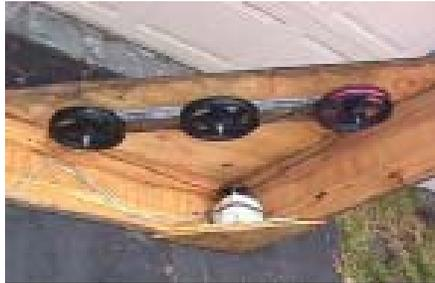
Problem was it becomes kind of expensive, inefficient, and messy with all the added motors, lines, and pulleys. To solve this I came up with a portable drive-unit that runs 3 separate paths/lines from one motor source.
