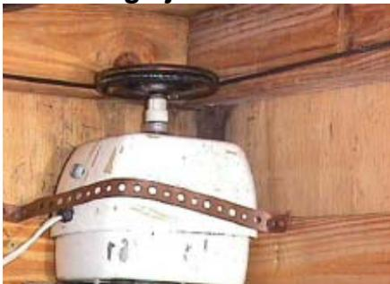
The orange juicer is not the only motor that can be used. Any electric motor with a shaft will work. I just happened to stumble upon an orange juicer at a garage sale and it worked out really good. It has great torque and the speed is fine. It could be a little faster, but then you might lose some control from the bouncing.
