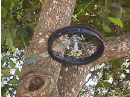
The larger hole on the strap's end is where you place the shaft of the bicycle rim and top it off by screwing on the nut.
