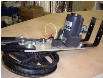
A co-worker salvaged this motor and gear reduction box knowing I would have a better use for it than the dumpster would. The final drive speed is about 60 rpm
