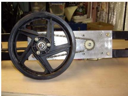
A piece of aluminum plate was used for the main chassis.
