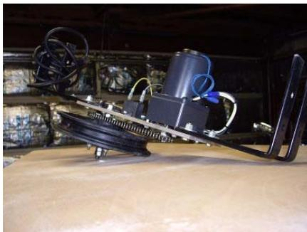
I had a length of #25 chain and a couple of 8" plastic wheels from a scooter, so with a quick check in the All Electronics catalog, I found the sprockets I needed.
