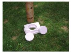
Cut 2 pieces of 2" Rigid foam slightly smaller than the top of your wooden box. Using your jigsaw, cut 2 8" round holes in the center of the foam. Glue the base pieces together with adhesive and then screw them together.
