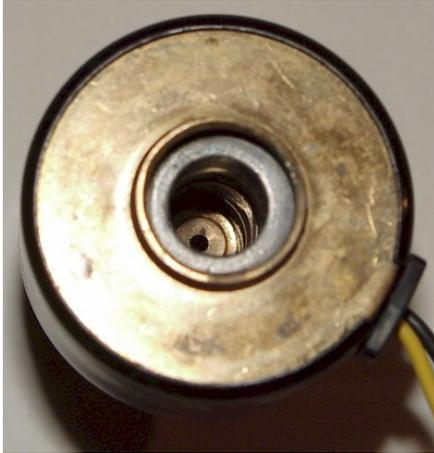
As you can see from the photo there isn't much to this tiny pump and only a few small rubber pieces. I don't know if vinegar would attack these pieces but mine were in good shape. On the left of item 1, this piece plugs into the little plastic tank on the fogger and inside of the black fitting is a screen.
