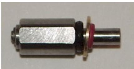
This is a close up of item 8. There is a rubber seal inside but you can see the little hole in the back. This is a very tiny hole and could clog pretty easily.
