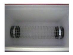
Here's the inside of the fog chiller. Basically two 4 inch reducers and some 0.5 inch hardware cloth clamped around the ends.
