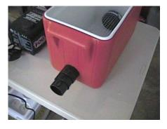
Output side. I put a female threaded coupler on the 4 inch reducer so I could screw in an assortment of attachments. I can add an extension of 4-6 ft of rigid pipe or a similar length section of flexible duct.
