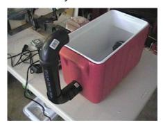
The intake side. A couple of elbows and a 8.5 inch length of pipe to get it at the right height for the fog machine to sit on top of the chiller. I did not glue the pipe in place so that I could also set the fog machine to the side of the chiller if I needed to hide it behind something low to the ground.
