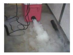
Here's the fog chiller in action. It's easy to construct and seems to do the job nicely. When I put the fog machine on full blast, the chiller doesn't make a whole lot of difference, but in short bursts (as shown in the image to the left) it works perfectly. If the fog machine was a bit smaller (lower output) I think the chiller would be perfect.
