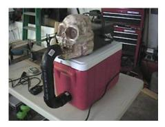
I did not seal the pipe to the fog machine. I do not want to risk having the end of the fog chiller outlet blocked by something and having pressure build up in the chiller. The fog machine expels the smoke with enough force to make it through the chiller without too much of it escaping back out the inlet. With the inlet higher than the outlet, the cold smoke tends to only go out through the outlet when the fog machine is re-
