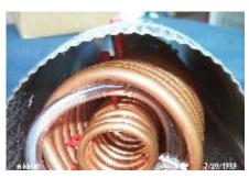
If you look closely, you can see how the coils are suspended inside the stove pipe. I used red plastic wire ties to connect the inner coil to the outer coil, and a second set of ties to connect the outer coil to the stove pipe.
