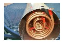
This is the other end of the chiller. The red caps came on the copper I bought. You remove them and that is where the plastic tubing is attached. I drilled some larger holes for the tubing to exit that you can just barely see on the top of the stove pipe.
