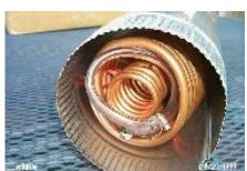
This is what the end of the chiller looks like. You can see the 1.5 inch inner coil and the 3 inch outer coil and the short plastic tube connecting them.
