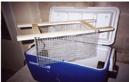
Now comes the most difficult step of the whole construction, building the cage that holds the ice. Cut two pieces of 1"x2" about 1/2" wider than the inside width of your cooler, then cut two more pieces of 1"x2" just long enough so you can fit the cage frame into the cooler.
