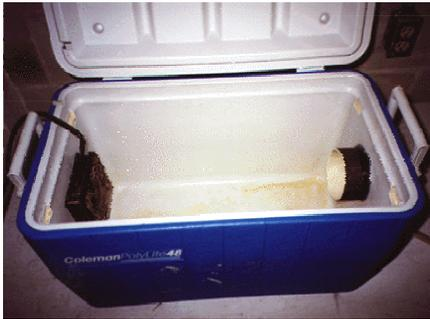
Install the 4" fan to the inside of the cooler that has the pipe flush with the inside wall. I used long skinny sheet metal screws to attach the fan. Be sure you have the fan facing the correct way so it is blowing out the pipe. On the other side of the cooler is where the fog machine will go so the fan sucks the fog through the chiller.
