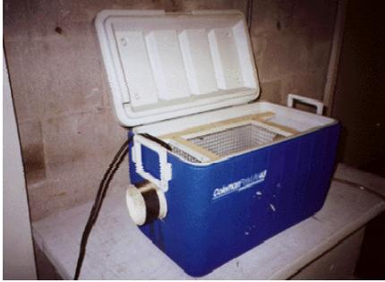
Here is the fog chiller that I built for a haunted house I work at. It is reliable, lightweight when empty and is very durable. I used a 48 quart cooler but you could use a smaller one if you wanted to. This chiller easily handles a fogger with an output of 7000 c.f.m. If you have a larger fogger than that I would suggest a 48 quart or larger for sure. Cut a 4" hole centered on both ends of the cooler with a hole saw just below the handles.
