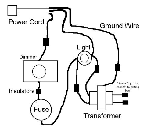
This diagram is with the power lamp and the drawing I used:
