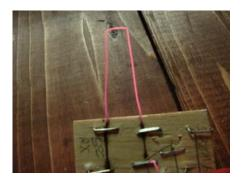
5) A longer wire requires more power then a short piece of wire so remember to turn your dimmer down when switching jigs. I have a habit of pressing the dimmer (which shuts the wire off) ,switching to a smaller jig, and tapping the dimmer on......needless to say, the wire glows orange and if I don't kill the power quickly the wire will break/melt. The second picture IS NOT what you want.
