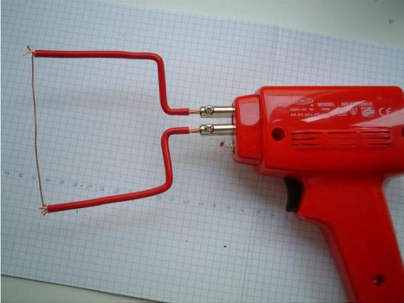
If you are concerned, you can compare the AC voltage (with trigger pressed) at the terminal posts with the new loop fitted, with the voltage when the original soldering loop was fitted. If the voltage with the new loop is the same or higher than the voltage with the original loop then the power taken from the gun is not more than its design value and it will not overheat.
