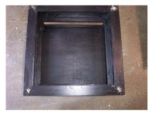
Using either scrap or new lumber, construct a box to house the fan and paint it black. Since the dimensions or the box will differ depending on the size of the fan, exact measurements are not given. Take notice of the small "lip" inside the box which supports the fan.
