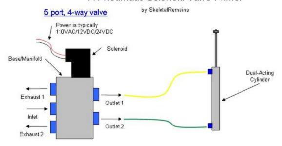
This is the other 4-way valve, the 5-port version. It is my solenoid valve of choice that I like to use everywhere because of it's flexibility. The only real difference here between this valve and the 4-port version is that there are 2 exhaust ports. Why on Earth would anyone care if the exhaust ports are combined or separated? Well, let's first look at flow-control, and then we'll come back to that question.
