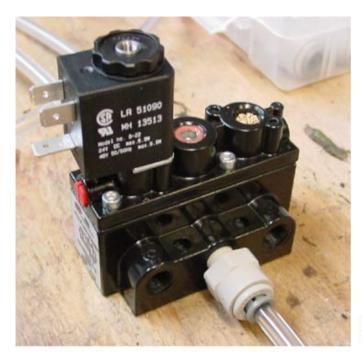
Valve for controlling dual acting cylinders (Grainger # 4XT32)
