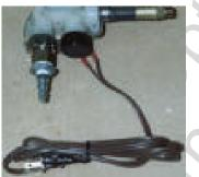
And here is how it will look when completed. The top of this photo got cut off, but you can see that 3/8" air hose slips perfectly over the outlet nipple for feeding the air to your prop. And that's it!
