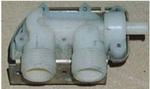
Of course you will need a water valve from a washing machine and not just any valve will hold the air back and reseat itself under the rather high pressure I would need for an air cannon. I wound up testing many, many different valves to see which work and which don't.
