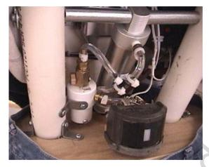
Here is yet another way to use your compact muffler. These photos, which was first used in the 2003 project, the <u>Lynching</u>, shows a second fitting on the top side of the muffler that can be used to silence the exhaust from the secondary air inlet on a 2 way air ram. You must route these two lines into the muffler separately, as if you link them together, you will in essence be attempting to force air into both the PUSH inlet and the PULL inlet of the same air ram.
