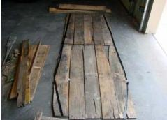
Use a reciprocating saw to cut off the nails from the pallets to separate the boards. This is a lot of work and you need a helper to hold up the pallet as you cut.
