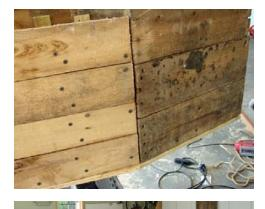
Now for the angle sides. Measure the distance from the end of the side to the header. Using your square, mark off and cut the side to fit.
