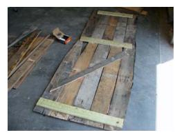
At the top, bottom and middle: slide a section of the fence post underneath. Leave a 2 inch space from all sides.
