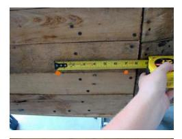
To make the rope handles measure and mark two holes 7 inches apart halfway up from the bottom of the coffin. Get it as close to the angled part of the coffin as you can.
