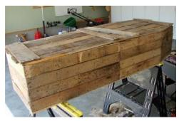
Measuring from the bottom plywood, mark the perimeter of the coffin 14 1/2 inches high. Cut this out with the circular saw.
