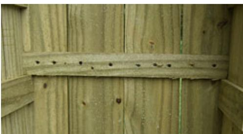
The remaining 23" and 18" sections of board #15 were used to secure the four boards that formed the bottom of the coffin.
