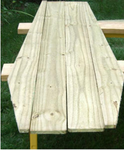
Boards #1, #4, #5 and #8 form the sides of the top and bottom of the coffin. These must be cut to achieve the toe-pincher angles. Marks were made two inches from one side on both the top and bottom edges. Another mark was made 16 inches from the top on the side opposite the other two marks. The marks were connected by a line which was used for the cuts. We ended up with two sets of four boards shaped like those in the picture on the right.
