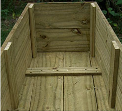
The vertical ribs were all glued and screwed to the sidewalls and foot section.
