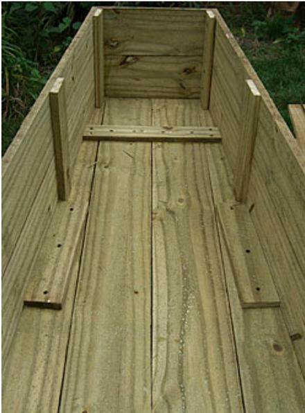
The 18" cross member from board #15 provided the sidewall support near the foot of the coffin. Therefore the two 10" sections of board #14 were not used.
