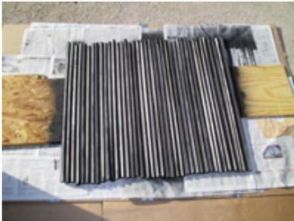
The pvc pipes are cut to 2 foot lengths I drilled holes in them about 6 inches from the top and bottom for the bolts to fit through.
