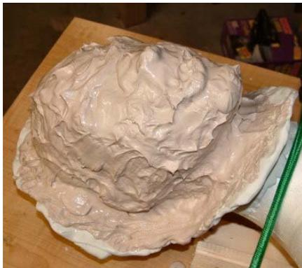
Mix your first batch of plaster in a large bowl or bucket to a consistency a little thicker than pancake batter. Coat the sculpture with hand soap to make de-molding easier. Brush on the first coat (called the detail coat). Make sure to spread the plaster over every surface. The plaster may slide off the face because of the soap. Don't worry. Just keep dabbing it on.
