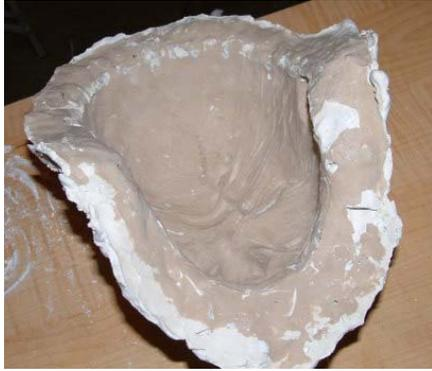
The mold you've just made is a negative image of your sculpture. What you've made is also called a one-piece mold. If you had been making a mold of the entire head including the area behind the ears, then you would have had to make a two-piece mold. I wanted to tackle one thing at a time before I invited extra frustration by complicating matters. That's why we're only doing the front of the head.
