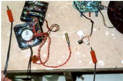
Here you can see the sound chip, which is a small black box that records any message for up to about 8 seconds and then will play it back when the little sensor (the brass tube) senses a change in heat. This particular one came from Terror By Design. We will be talking about this in a moment. The same as we did when modifying the Boris head for the Crypt Keeper, we will once again be cutting off the microphone and soldering our inline electronics to the center wire.
