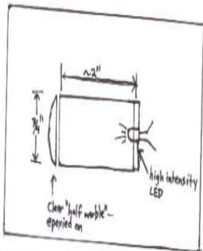
How about some really scary led eyes? Dinky little red led's on this impressive prop would have looked dorky. So, I came up with a way to generate LOTS of light for the eyes with the high intensity LEDs. Just make a bit of a magnifying glass.
