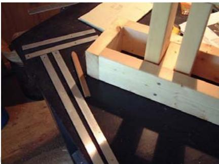
Cut two 30" and 7" pieces of aluminum stock. Drill holes at the corners, while leaving an extra 2" overhang on the 7" pieces (fig. 5). Use the 5/8" #8 bolts, washers and nylon lock nuts to assemble the mechanism, do not over-tighten.
