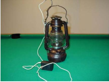
Here is a standard lantern available at any hardware store. I cut off the bottom, installed a flicker circuit, a 9v battery eliminator, a bulb socket, and bulb. I then used a plastic cup and some fiberglass to seal up the lantern. A little black and brown paint and here is the old looking lantern
