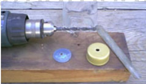
Start by removing the plastic seal (ours was blue) from inside the lid with needle-nose pliers, the glue won't stick to it very well. Now carefully drill a hole the same diameter as your clear tubing through the center of the cap. Remove any plastic debris from the drilling, then lightly sand both the inside and outside the cap around the hole to help the glue stick to the plastic better. An emery board works great.
