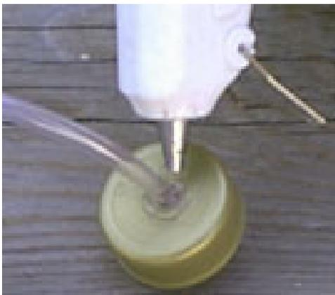
After allowing the glue-gun to heat up to operating temperature, push one end of the plastic tubing through the hole until about a quarter of an inch sticks out from inside the cap. Carefully use the hot glue gun to thoroughly seal the tubing in place by surrounding the gap both inside and outside the cap. You can use plenty of glue on the inside as it will not show. While the glue is drying on the cap you can bend the bailing wire to make the wire for the hanger part of the bottle.
