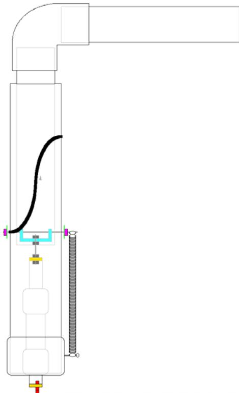
As the piston pushes forward, the metal bar rides in the spiral shaped slot. This causes the 1.5 inch pipe to twist and raise. It does this with considerable force. I fitted an elbow and another 12 inch piece of 1.5" PVC pipe to the end of the inner PVC to form the arm. It swings it with enough force that I decided to get some thin wall PVC (instead of the schedule 40 I used everywhere else) so that it was lightweight enough that if it hit anyone, it would not hurt them.
