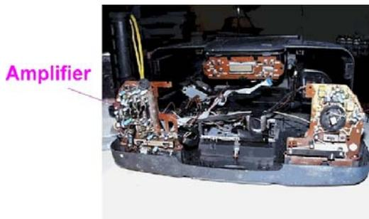
For our first way to make this old boombox into an amp, we will be using the part previously used by the radio.
