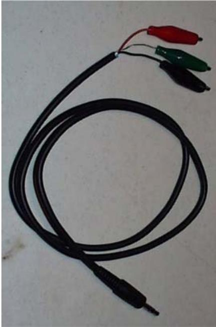
Now that we have found the left and right channels we just need to find the audio common wire. In some cases it could be the same as the common ground which seems to be so in this case.
