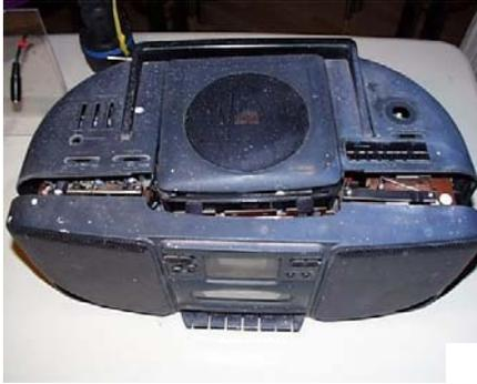
"In this first picture I show you what to look for. This type of radio is the simplest to modify into an amplifier if you are looking to use a radio boombox. However, if you have a radio with a single PCB, (printed circuit board) you can still use this same process. It is just a bit harder to determine where to tap into. More about that later.
