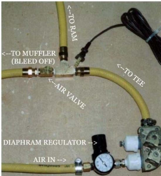
Here is an old photo of the completed system (using the previous method of forcing the PVC pipe end caps on which were tapped with threads for the air fitting) put together for the [Exorcist](#) that illustrates well how this will be used.
