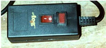
I open the switch box up and test the two leads connected to the switch to see if they carry current while the circuit is closed ("closed" meaning when the circuit or wire is fully connected in a continuous manner with no breaks as it would have when the switch is not being depressed) using a 110 V meter.
