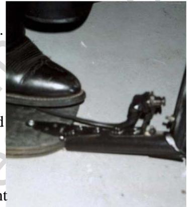
The other end of the short 5" to 6" section is attached to the wood platform with another hinge. Notice that this hinge is only attached to the board with one screw and even that one is not tight. This attachment is loose on purpose.
