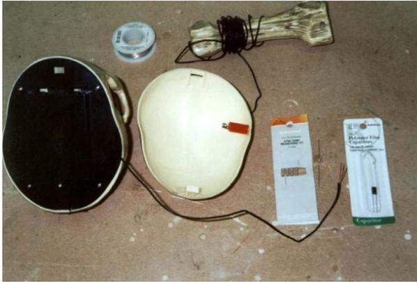
After a great deal of help from the folks on the [chat list](#) I was able to find a capacitor and resistor that would allow me to use the headphone out jack on my cassette player to send a signal to the line that the microphone attaches to on the Boris. Radio Shack carries this .01pF Polyester Film Capacitor and the 10K ohm resistor you will need. The photo above shows a picture of a 470 k ohm resistor, but it turned out that the correct one is the 10k, so substitute the 10 instead.
