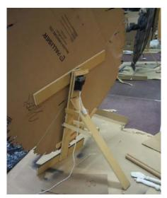
The base was thrown together together with 1x4's and 1x2's. I drilled a hole for the business end of the motor to poke through, which also took it through the lazy susan, and bolted it to the 1x4 on the other side. Sorry, but I don't remember how I managed to pull that off. I just remember it got a little tricky.
