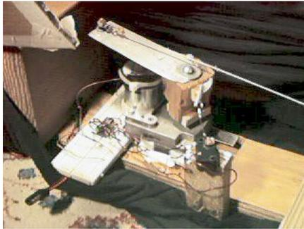
The metal lever rotates freely on the wooden base which is attached to the motor. As the base rotates, a screw sticking up from the base catches the lever and pulls it around raising the Flailer's arm. The motor is stopped just short of pushing the lever all the way around. To release the arm, the motor simply starts running again and pushes the lever past the critical point. Then the lever is pulled around, away from the screw, by the arm's elbow springs.
